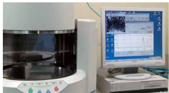
蛍光X線分析器(RoHS指令用分析器) X-ray fluorescence analyzer (RoHS analyzer)
